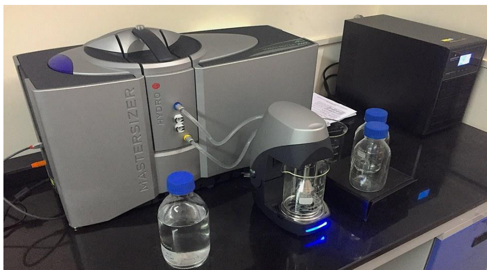
Figure 2: Grain Size Analyzer (Malvern Mastersizer)
