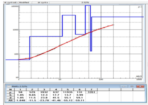
Figure 2: The model fit is exhibited by the curve of the Schlumberger depth sounding at Site A, which is of A-Type.
