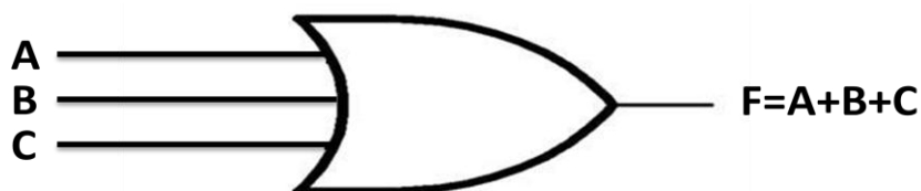
Fig.2.2 A 3 input OR gate
