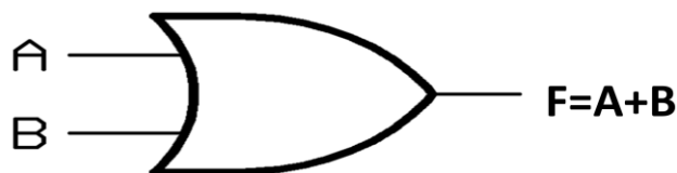
Fig.2.1 A 2 input OR gate
